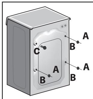
Remove the screw (C). A spacer will fall inside the machine.
